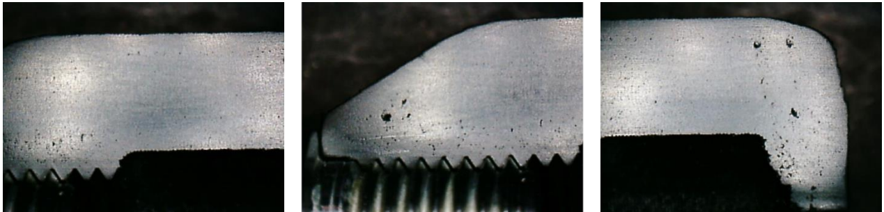
Image 2: Micrographs of the 3D-printed clutch hub
